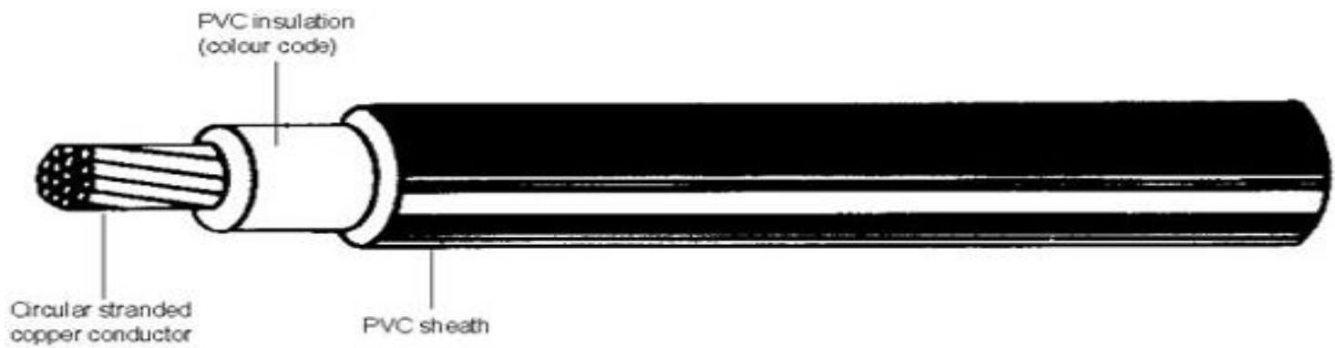
Single, circular stranded copper conductor, unarmoured, sheathed cable
